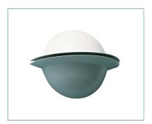
The CTVK is a very quiet supply air diffuser designed for wall mounting. The diffuser is suitable for use in small premises, such as offices, houses and hotel rooms. The air discharged from the valve is mixed thoroughly with the room air thus providing a draught-free air supply. The air flow is adjustable.
